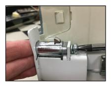
**Step 2:** Remove the old lock and/or housing by removing the pan head screw from the rear of the lock. Keep the screw and lockwasher for re-use.
