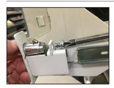
**Step 3:** Remove the old lock and/or housing.
