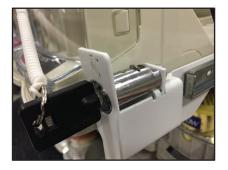
**Step 1:** Unlock the unit and open the tray to access the locks.
